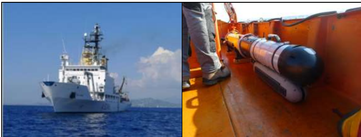
Figure 5: (left) CMRE’s research vessel: the ALLIANCE, (right) REMUS equipped with the UWBS system on the dock of the small boat ready to be deployed.
