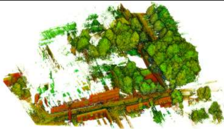
Figure 12: Kings Building scans using VUX-1LR and custom backpack system developed by us.
