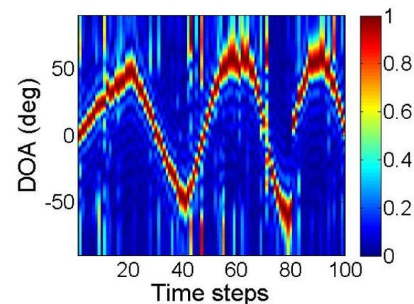
Figure 2. Narrowband DoA estimations for moving source (SNR=20dB), 22/100 active sensors
