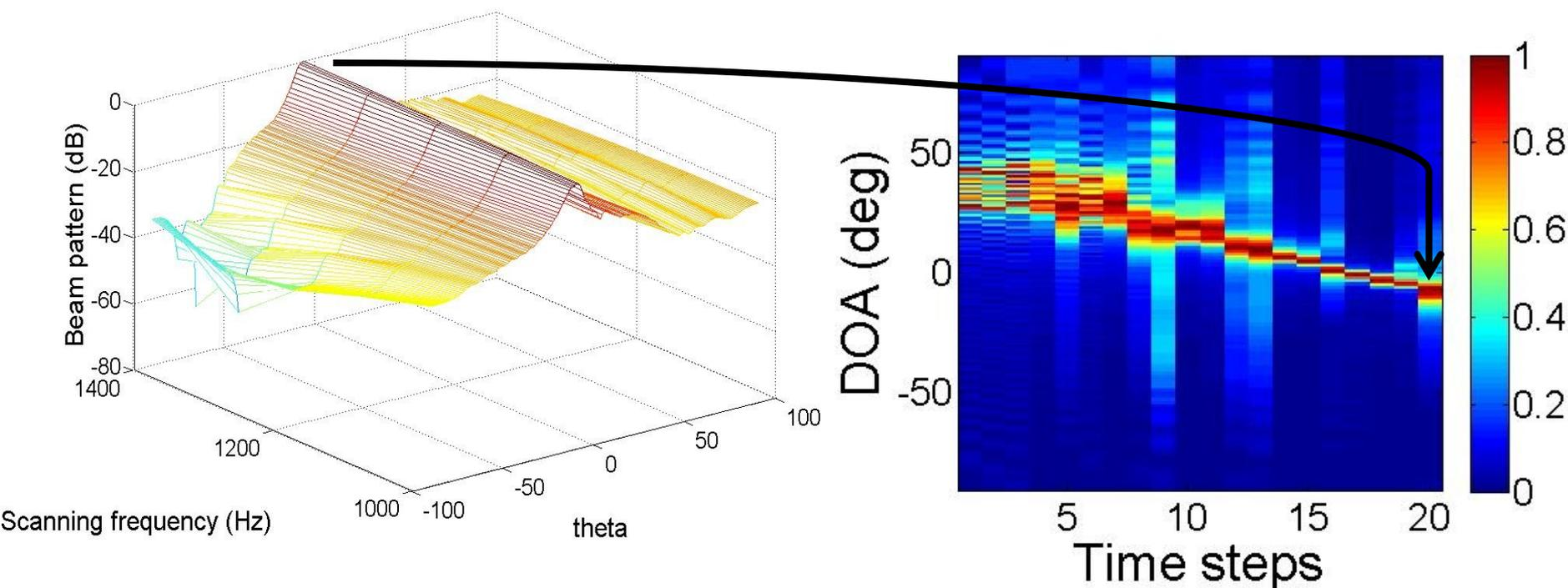
Figure 3. Wideband DoA estimations for the moving source, the 3D graph illustrates the simulation result at the 20-th time step and the spectrogram is the DoA estimation for the last frequency band, 69/300 active sensors.
