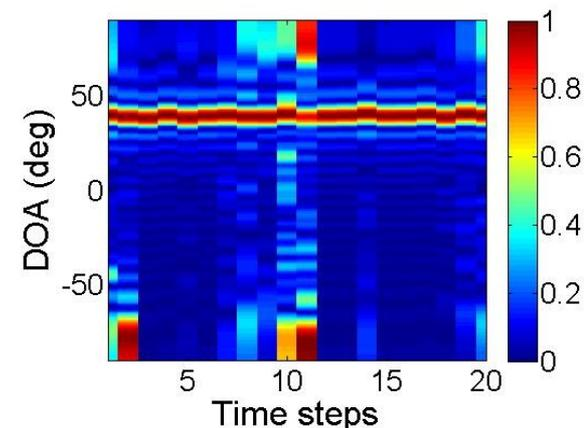
Figure 1. Narrowband DoA estimations for stationary source (SNR=20dB), 37/100 active sensors
