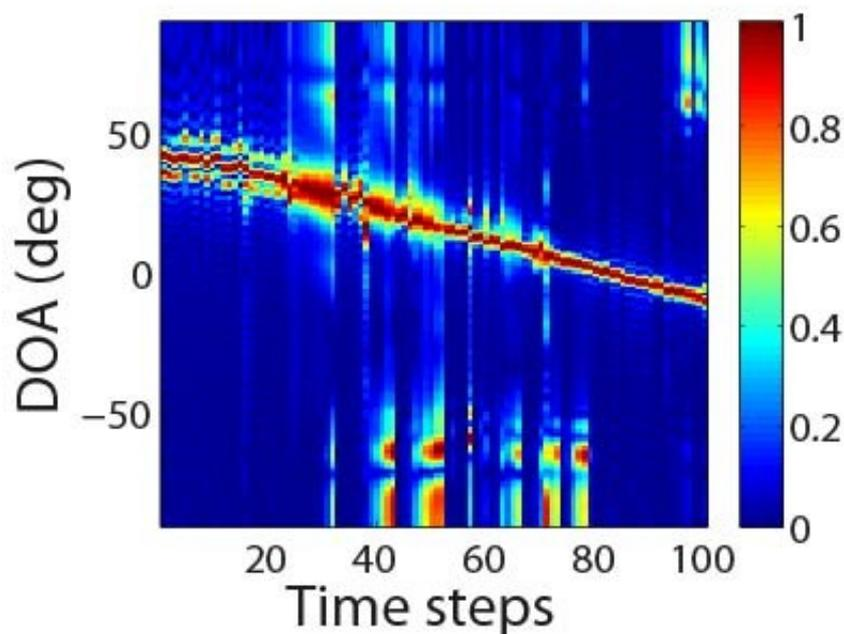
Figure 5. DoA estimated for the moving source without noise at the frequency band of 1100 Hz, 59/300 active sensors
