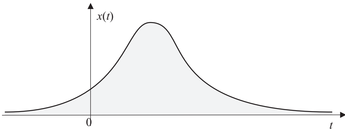
Figure 1.4: An example of an aperiodic signal.
