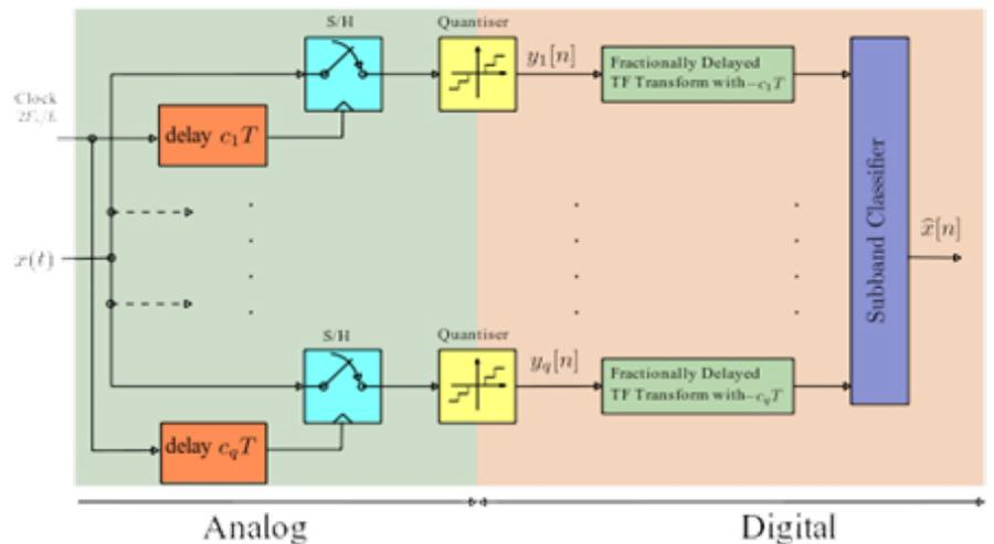
LoCoMC is suitable for SWAP implementation, as it needs only a few ADCs and synchronization of ADCs is possible in digital domain. The benefits of using LoCoMC over other sub-Nyquist methods are:
