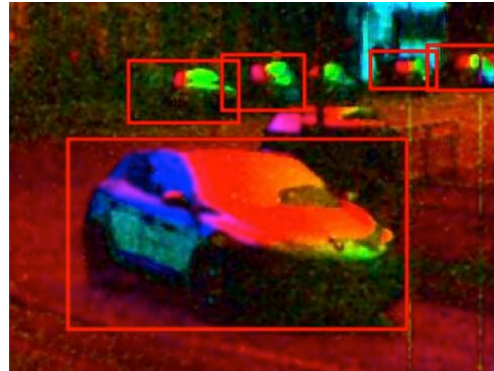
vehicle detection using polarised infrared sensors [Sheeny 2018]
