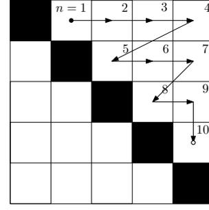
Fig. 1. Values of  $n$  used for cyclic-by-row sequence of Jacobi rotations in one Jacobi sweep for a  $5 \times 5$  matrix with start  $\bullet$  and end point  $\circ$ .
