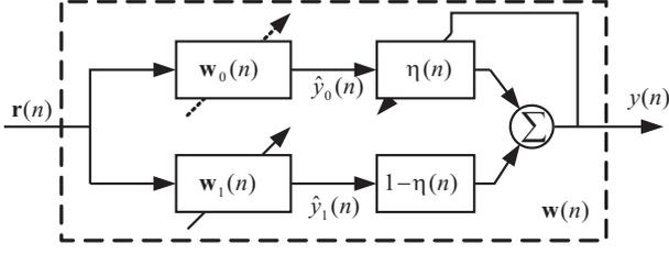
Fig. 2. Diagram of the proposed KA-STAP algorithms. The upper-branch filter  $\omega_0(n)$  is fixed in the LCICM scheme and adaptive in the MLCICM scheme. The lower-branch filter,  $\omega_1(n)$ , is adaptive in both schemes.
