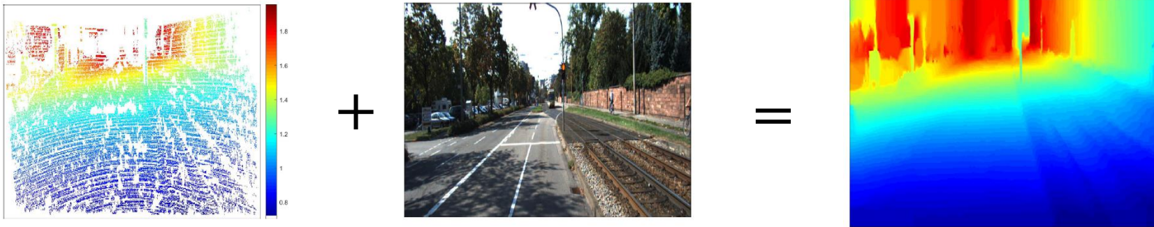
Fig. 1. Diagram of our method. Given an RGB image I and LiDAR data L , it generates a vector u that is used as side information in the optimization problem. The output is a dense depth map \hat{x} .
