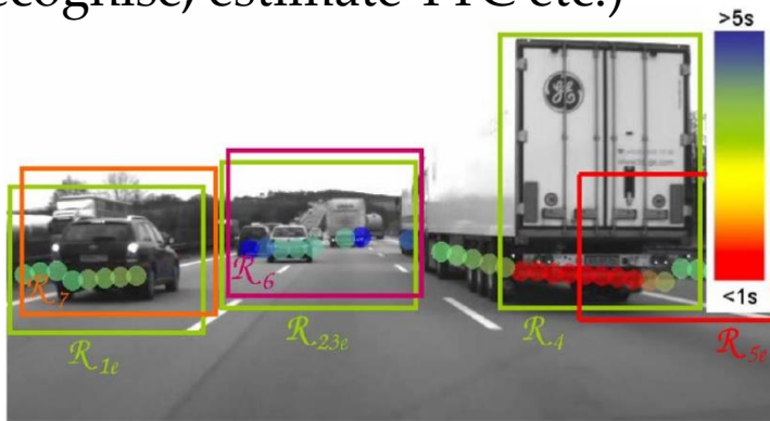
Fig. 15. TTC values for the example road traffic scene. The minimum TTC inside each region is used as t_{TCC} and drawn in HSV color space.
