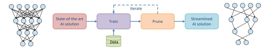
Demonstrator result: 90% less computations; 99% less memory ⇒ Only 3% reduction in accuracy
