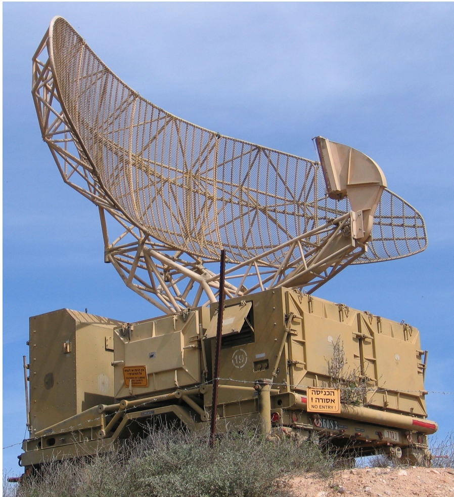
Figure 2.5: Radar of the type used for detection of aircraft. It rotates steadily sweeping the airspace with a narrow beam. Air Force Museum, by Bukvoed / CC BY-SA 3.0.
