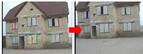
Figure 5. Example scene rectangles (left) and identified building apertures (right)
