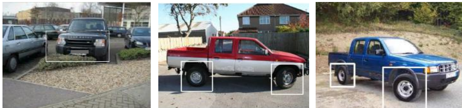
Figure 4. Example part-wise vehicle detection in visible-band imagery under varying poses.
