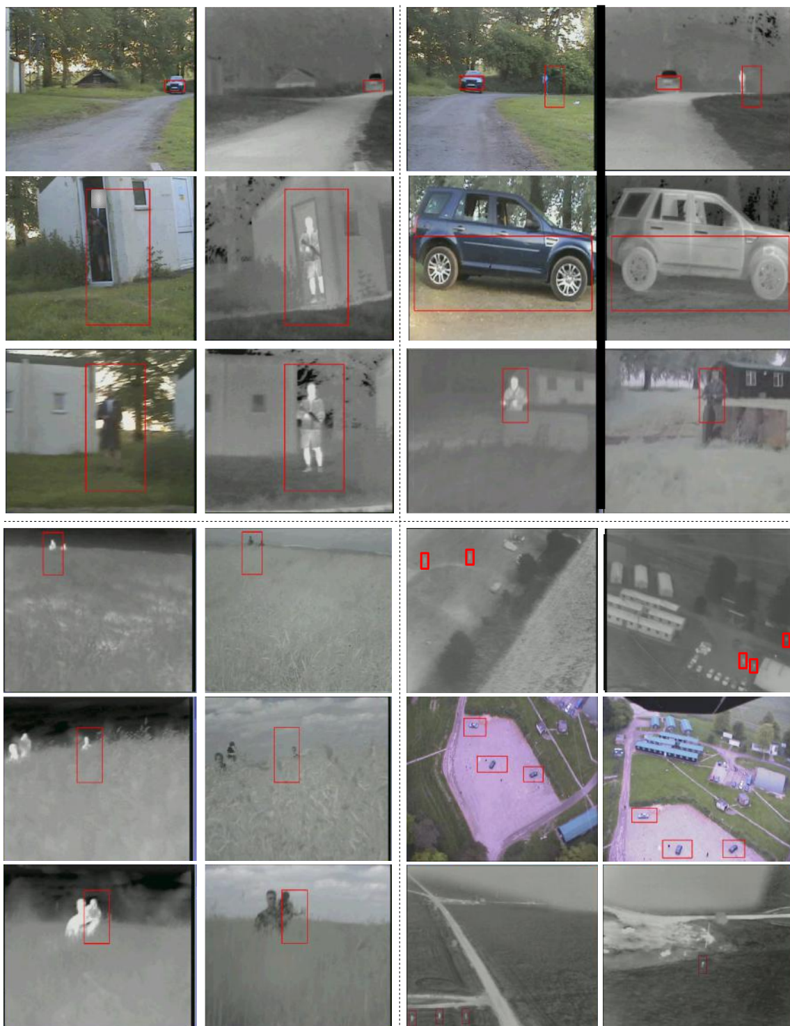
Figure 12. A range of both ground and aerial targets detected over Evaluation Trial 2, presented in {visible, thermal} imagery pairs as appropriate (UGV ground detection examples, top right/left and bottom left) and visible/thermal imagery only (UAV aerial detection examples, bottom right).
