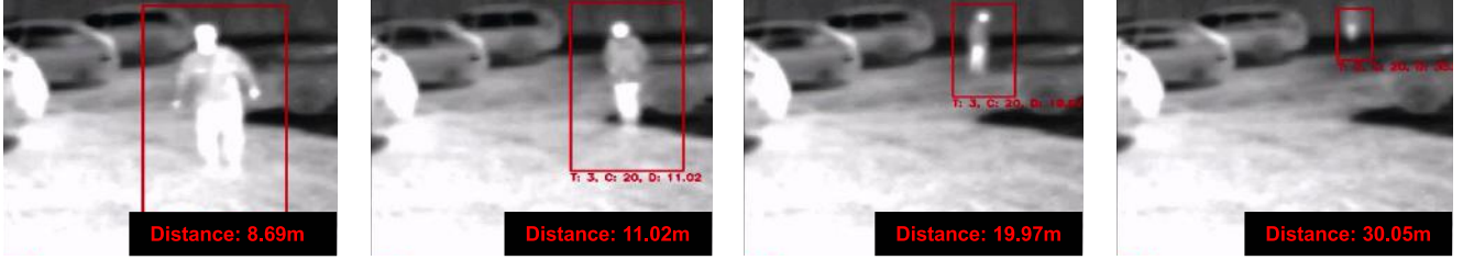
Figure 9. Photogrammetry facilitates the approximate recovery of a sensor to target distance for an example target (person) without any need for additional (active) range sensing.
