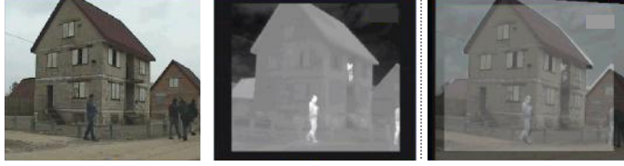
Figure 8. Visible-band image (left), thermal-band image (middle) and resulting image registration (visible-thermal overlay) (right).
