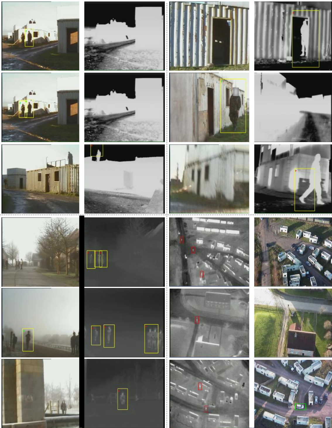
Figure 15. A range of both ground and aerial targets detected over Evaluation Trial 3, presented in {visible, thermal} imagery pairs as appropriate (UGV ground detection examples, top right/left and bottom left / UAV aerial detection examples, bottom right).
