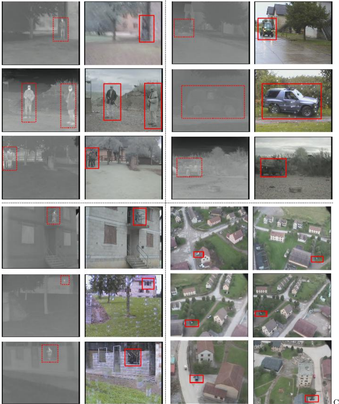
Figure 11. A range of both ground and aerial targets detected over Evaluation Trial 1, presented in {visible, thermal} imagery pairs as appropriate (UGV ground detection examples, top left/right and bottom left) and visible imagery only (UAV aerial detection examples, bottom right).
