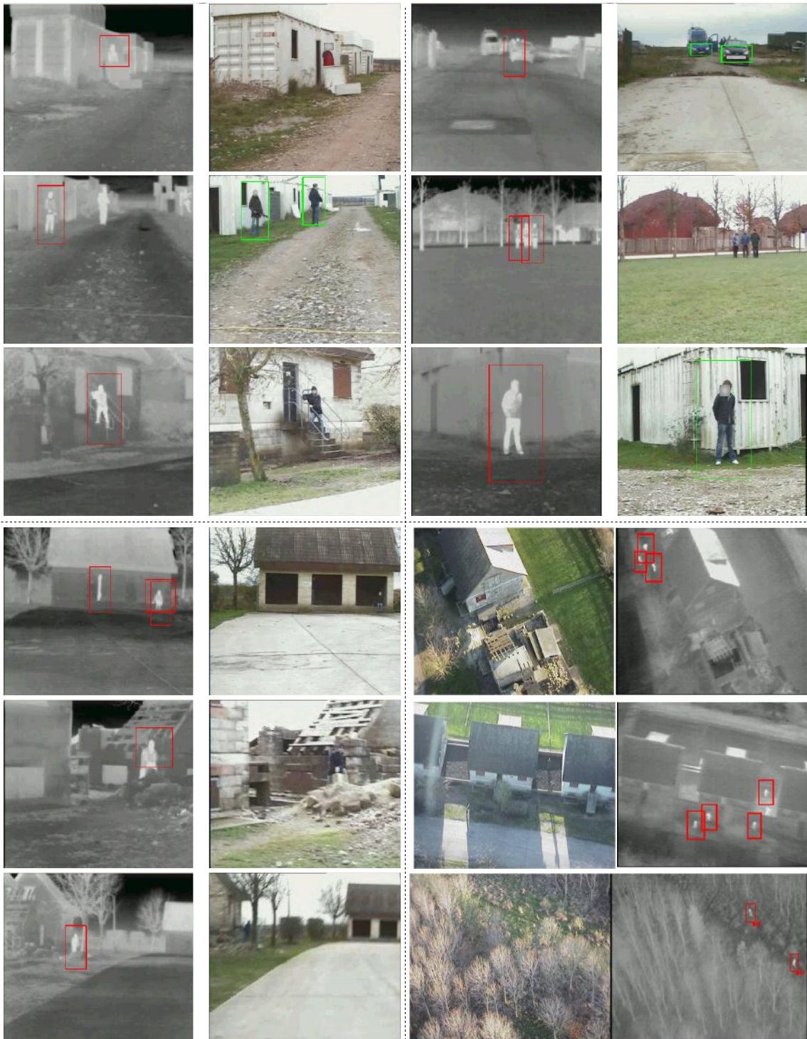
Figure 14. A range of both ground and aerial targets detected over Evaluation Trial 3, presented in {visible, thermal} imagery pairs as appropriate (UGV ground detection examples, top right/left and bottom left / UAV aerial detection examples, bottom right).
