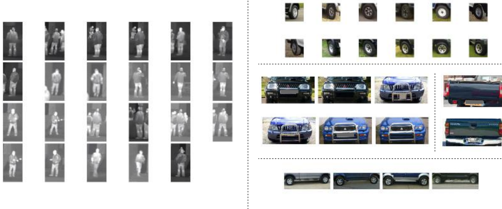
Figure 3. Example labeled training data examples for thermal-band people detection (left) and visible-band vehicle sub-part detection (right)
