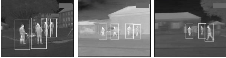
Figure 2. Example people target detection in thermal-band imagery under varying ambient thermal conditions.
