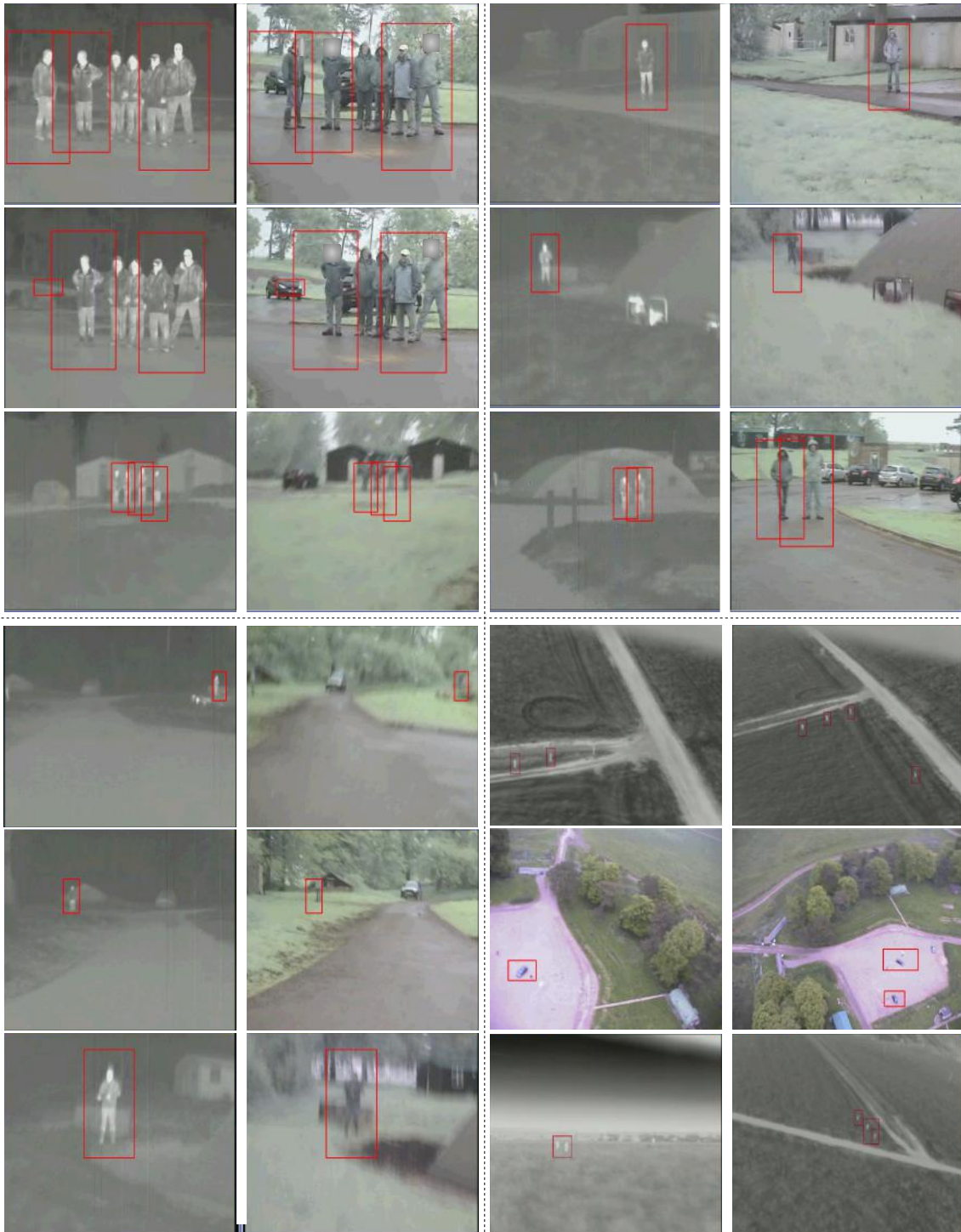
Figure 13. A range of both ground and aerial targets detected over Evaluation Trial 2, presented in {visible, thermal} imagery pairs as appropriate (UGV ground detection examples, top right/left and bottom left) and visible/thermal imagery only (UAV aerial detection examples, bottom right).
