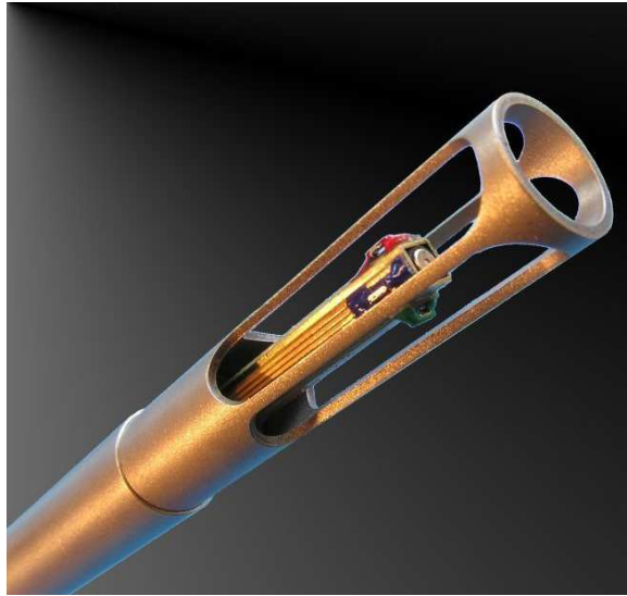
Figure 7.6: An acoustic vector sensor.
