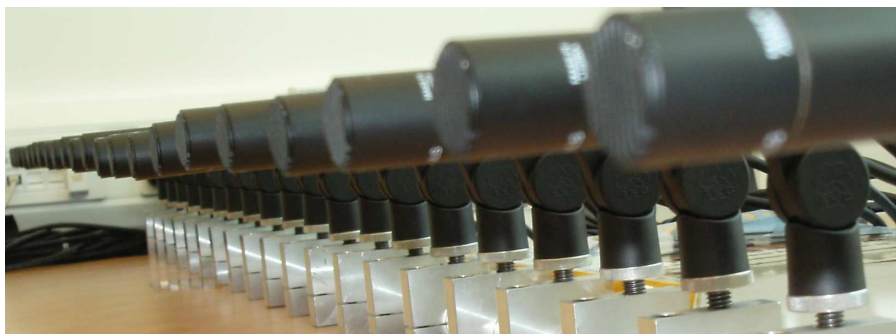
Figure 7.5: An ULA of microphones.
