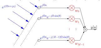
to steer the array characteristic towards this source, the output
