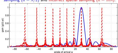
MIMO systems perform beamforming, but may dissipate energy into aliased directions.
