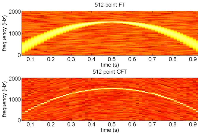
Fig. 2. A comparison between the FT spectrogram and the ppCFT for the signal  $\exp(2\pi i(-2048t^3 + 3072t^2))$  in Gaussian white noise ( $f_s = 4096$  Hz). The spectrograms are computed using a Hanning window of length 512 points and overlapped by 87.5%
