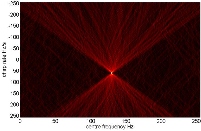
Fig. 1. Image of the CFTs using the full range of chirp rates, for the signal  $\exp(2\pi i(30t^2 + 130t))$  in Gaussian white noise.
