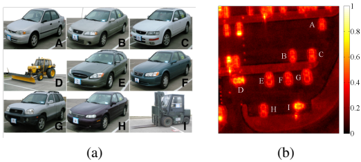
Fig. 3. GOTCHA Dataset: (a) images of the vehicles used as targets; (b) full-azimuth and full-polarimetric magnitude SAR image of the area of interest containing the 9 vehicles.
