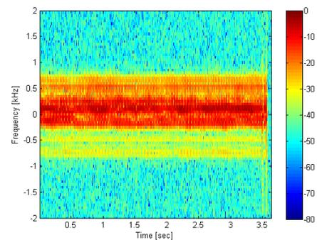
Fig. 6. Micro-Doppler signature of a propeller, facing the array of microphones and the loudspeaker, ensouffled with a 20 kHz constant pulse.
