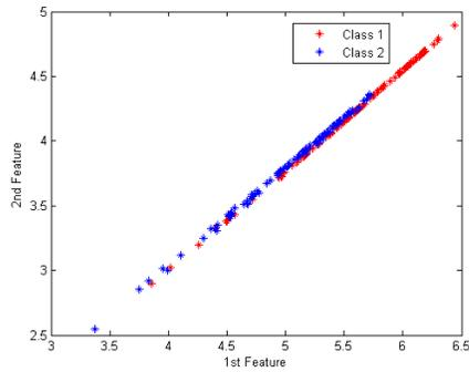
Fig. 7. MEL-Cepstrum feature extraction. Feature 1 versus Feature 2 for Target A (blue) and propeller (red).
