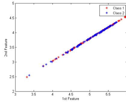
Fig. 5. MEL-Cepstrum feature extraction. Feature 1 versus Feature 2 for *Target A* (blue) and *Target B* (red).
