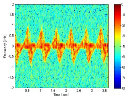
Fig. 2. Micro-Doppler signature of *Target B* at 20 kHz.
