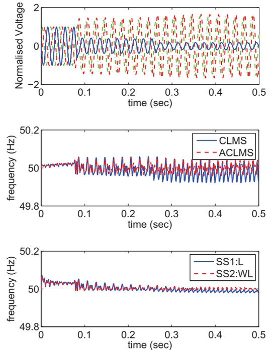
Fig. 4. Frequency estimation for real-world unbalanced three-phase voltages, where an initially balanced system experienced a single-line short with earth.
