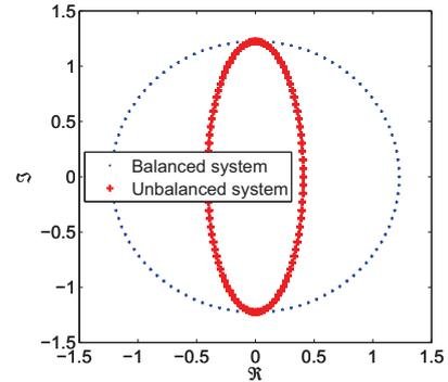
Fig. 1. Geometric view of circularity via a real-imaginary scatter plot of the output voltage  $v_k$ . For a balanced system, characterised by  $V_{a,k} = V_{b,k} = V_{c,k}$ , the trajectory of  $v_k$  is circular (dotted circle), while, for unbalanced systems, such as the 100% single-phase voltage sag in phase  $v_{a,k}$  illustrated by the ellipse in the figure (+), the trajectory becomes noncircular.
