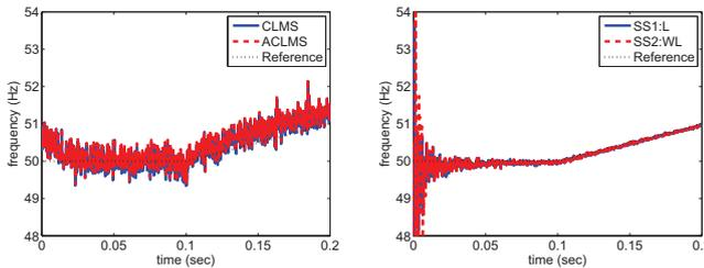
Fig. 3. Frequency estimation for a balanced system that experiences a 10Hz/s frequency rise starting at time 0.1s, all in the presence of white Gaussian noises at 25dB SNR.
