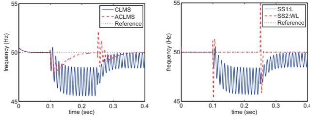
Fig. 2. Frequency estimation for a system which is balanced up to 0.1s, after which the system becomes unbalanced due to the occurrence of voltage sags of differing natures.
