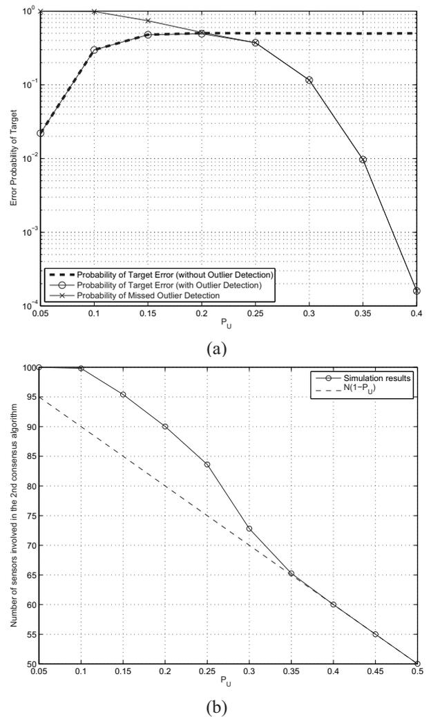
Fig. 2. Performance of the distributed detection with/without outlier detection for different values of  $P_U$  (Target SNR = 3 dB and  $A = 10$ ): (a) error probabilities; (b) the number of sensors in the second run of the iterative distributed algorithm.
