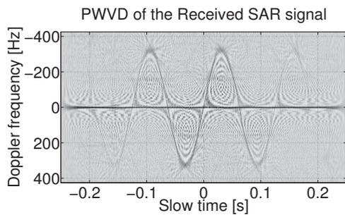
**Figure 2:** Pseudo-Wigner Ville Distribution of the analyzed range gate for the first simulated config.
