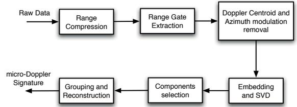
**Figure 1:** Proposed micro-Doppler extraction process.
