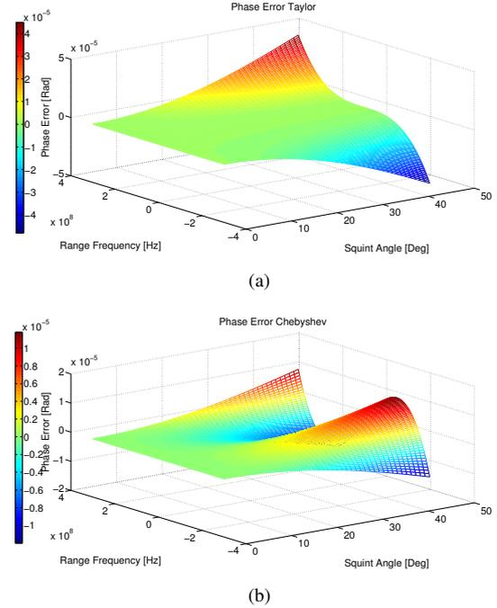
Figure 2: Phase Error for the spaceborne onfiguration for the a) Taylor and b) Chebyshev case.
