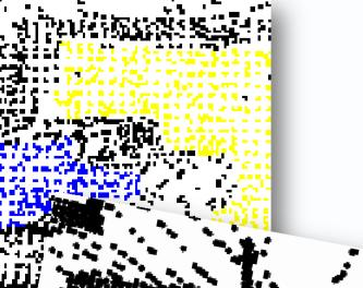
Shape based clustering. Points Are grouped into: clutter, target and non-target
