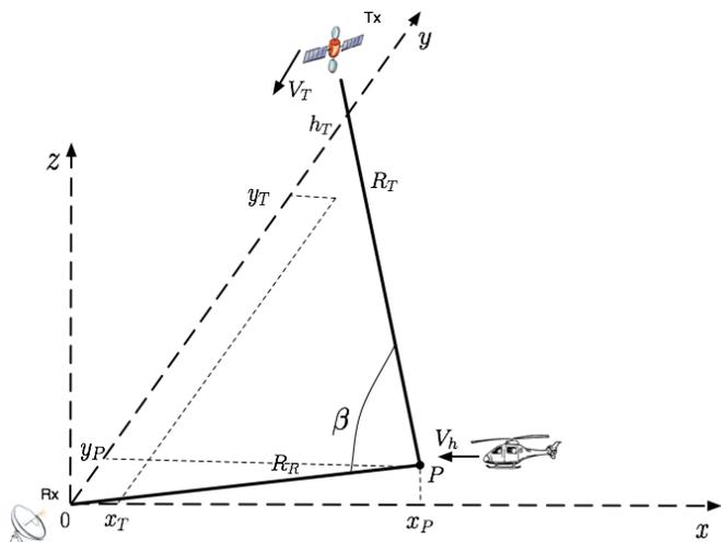
Figure 1: Proposed bistatic passive radar geometry with the GNSS illuminator.
