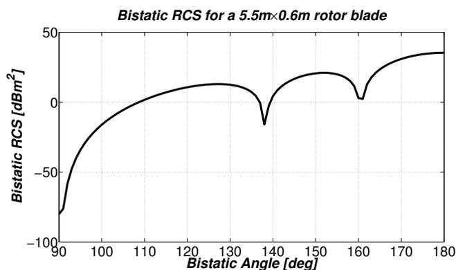
Figure 2: Bistatic RCS for a  $5.5 \times 0.6\text{m}$  rotor blade.
