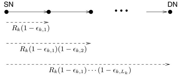
Fig. 3. The channel capacity for a serially connected path (as the first node has the highest capacity among all the nodes on the path, this node becomes the best node to be the EN).
