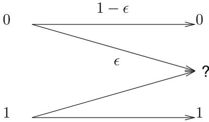
Fig. 1. Binary erasure channel model (in the figure,  $\epsilon$  denotes the erasure probability and ? denotes the erasure state).
