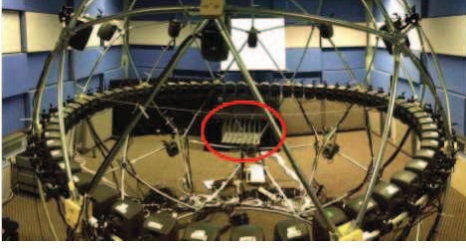
Fig. 5. Photograph of the experimental system showing the circular loudspeaker array and microphone grid (circled).
