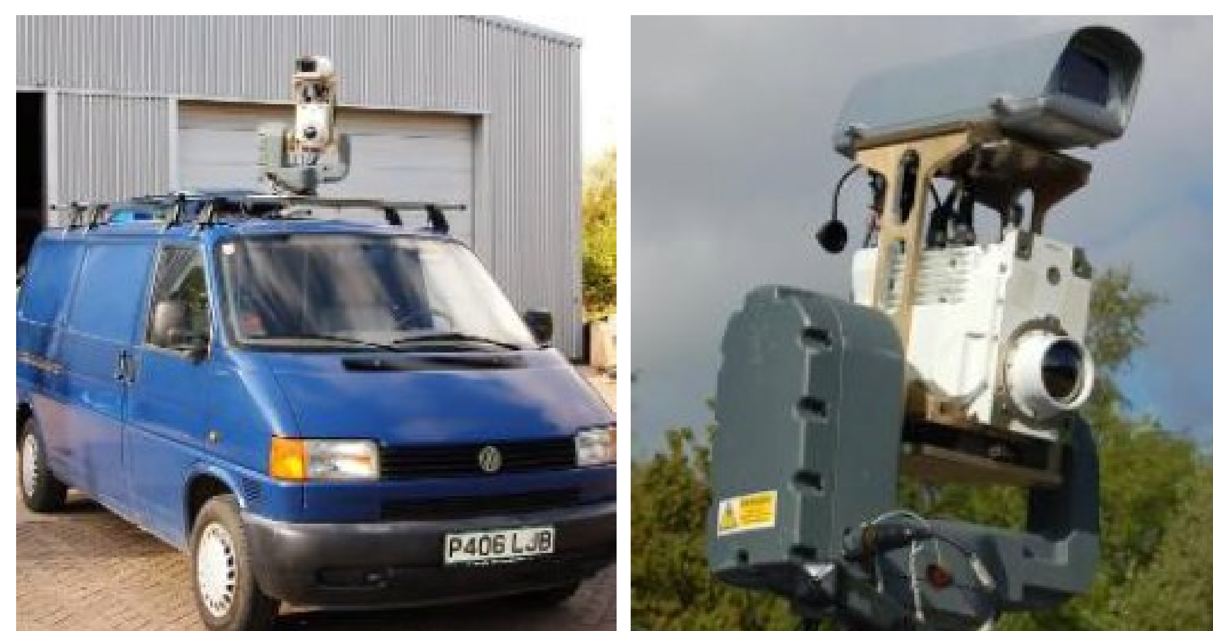
Fig 4: A ground vehicle (left) at Thales equipped with IR polarisation and imaging sensors (right).
