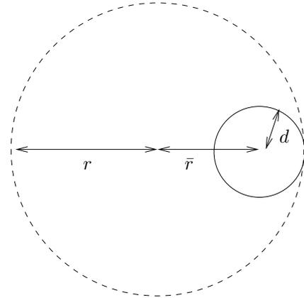
Fig. 2. The whole sensing area that is represented by a circle of dashed line and a sensing area of an LFC that is represented by a circle of solid line.
