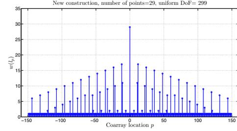
Fig. 4. The values of weight function  $w(l_p)$  given in the proposed CARS structure, as well as the maximum contiguous segments  $\mathbb{U}$ .
