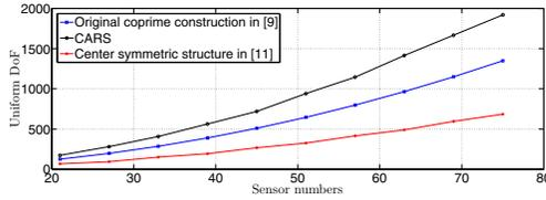
Fig. 5. Number of sensors vs uniform DoF for CARS, Original coprime construction [9] and center symmetric structure [11].
