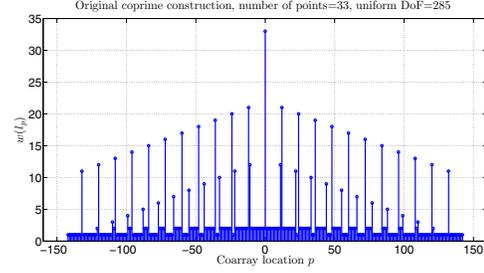
Fig. 3. The values of weight function  $w(l_p)$  given in co-prime structure in [9], as well as the maximum contiguous segments  $\mathbb{U}$ .
